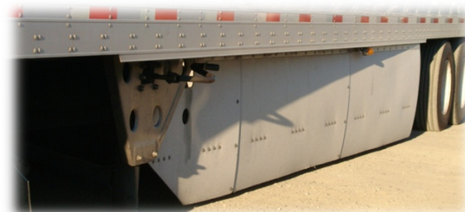
FreightWing Aeroflex skirts on Gordon Trucking trailers
